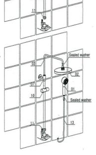
· Check up every step to ensure the stability and tightness to avoid any leaking before testing the shower spray.
